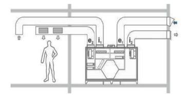
i1 (ETA) = extract air filteri2 (EHA) = exhaust aire1 (ODA) = outdoor air filtere2 (SUP) = supply air
