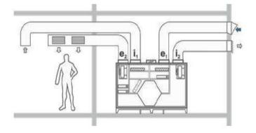
i1 (ETA) = extract air filteri2 (EHA) = exhaust aire1 (ODA) = outdoor air filtere2 (SUP) = supply air
